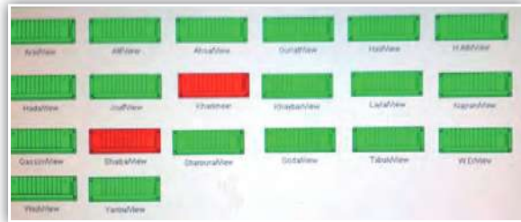
View (1): Clicking on one of the stations in red will reveal view (2) which shows the status of the building units (boards) of the faulty station following the same color scheme
