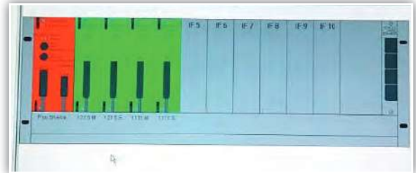
View (2): Based on this view, the SME will dispatch a maintenance technician equipped with a replacement board to that shown in red
