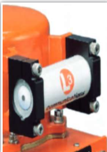
A close-up of an underwater locator beacon
