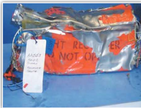
The damaged flight data recorder from Egypt Air Flight 990
